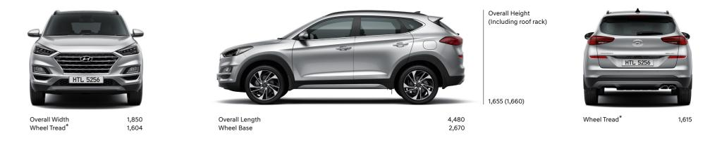
Unit : mm \* Wheel tread • 17" Steel Wheel, Alloy Wheel (Front/Rear) : 1,608/1,620 • 18" Alloy Wheel (Front/Rear) : 1,608/1,620 • 19" Alloy Wheel (Front/Rear) : 1,604/1,615
