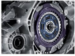
7-speed Double Clutch Transmission (DCT)
