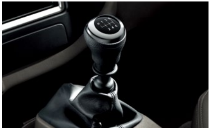
6-speed manual transmission Mated to the 2.5L engine, the all-new six-speed is noticeably quieter. Most importantly, the fifth and sixth overdrive gears will help conserve fuel and reduce your driving expenses.
