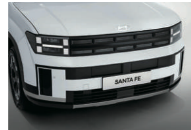
Radiator & Intake Grille
