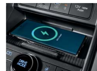
USB-C Data/Charging ports /Wireless charging pad
