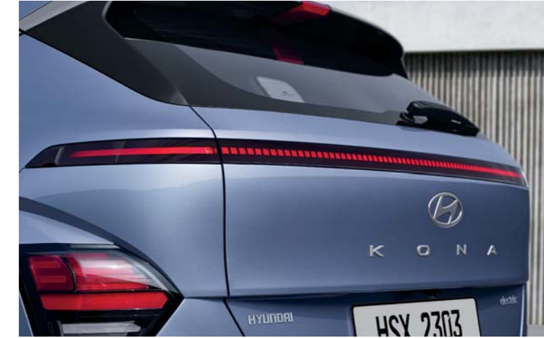
Rear pixelated seamless horizon lamp / Spoiler Integrated HMSL
