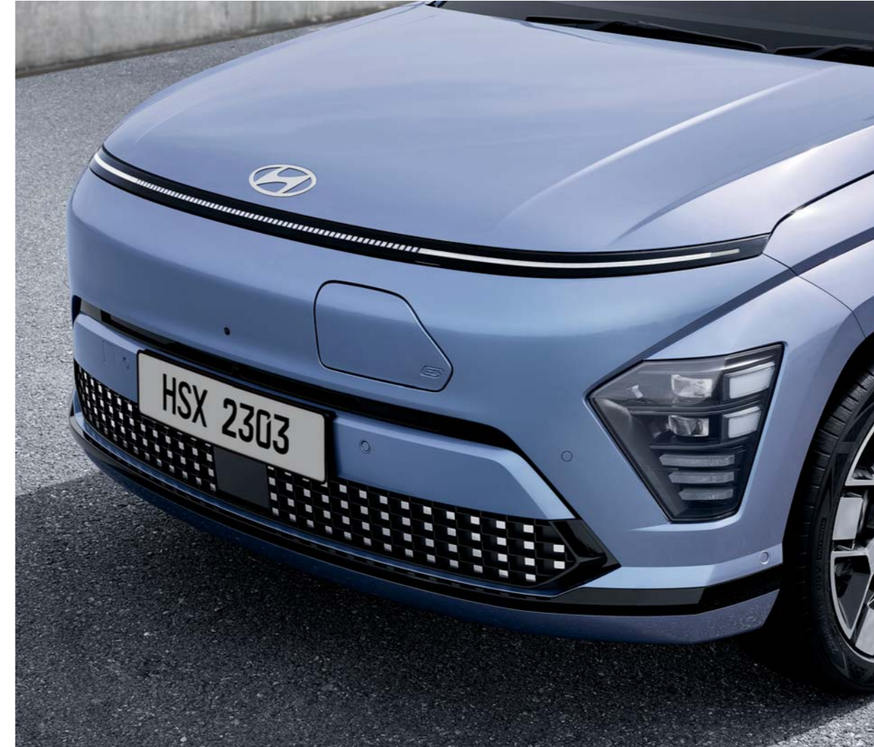
Front pixelated seamless horizon lamp (DRL) / Full LED headlamps (projection type)
