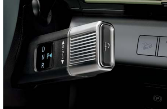
Column-Type Shift by Wire (SBW)
