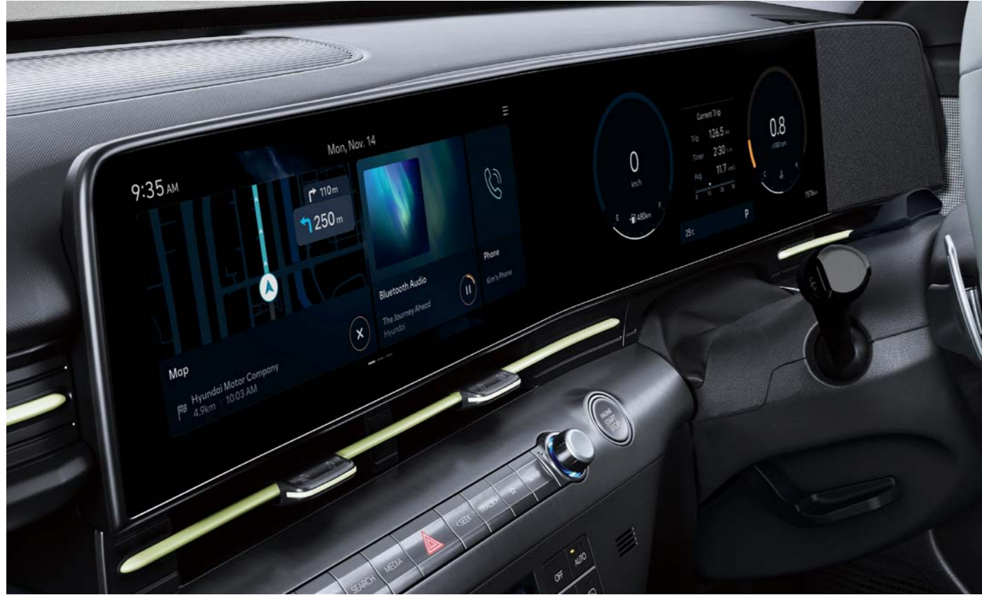
Panoramic display - 12.3-inch integrated dual screen display
